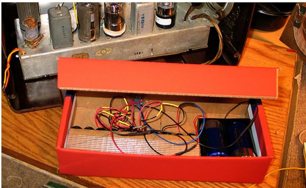
**Figure 6. AB Battery installed in radio. Cell holders and snap connectors are available at Radio Shack.**
